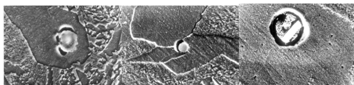
Fig. 2 – Complex REE oxysulfides in 09G2FB steel with 0.06% Y and microprobe points: a) – light part of the inclusion; b) – between the light and dark parts
