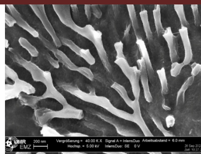
c. Fibrous eutectic morphology in Li0 HPDC alloy
