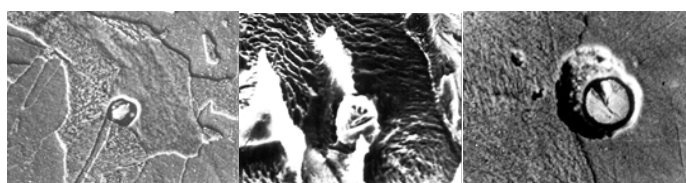
Fig. 4 – REE oxysulfides in 17G1SU steel with SIITMISH-1 additive (calculated for yttrium): a) – 0.05% (x1100); b) – 0.06% (x5000); c) – 0.07% (x2500)
